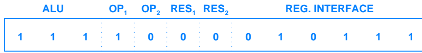
Figure 8.11 An example instruction that simultaneously continues an ALU operation and loads the value from register seven into operand hardware unit one. Horizontal microcode makes parallelism easy to specify.
