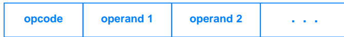
Figure 5.1 The general instruction format that many processors use. The opcode at the beginning of an instruction determines exactly which operands follow.
