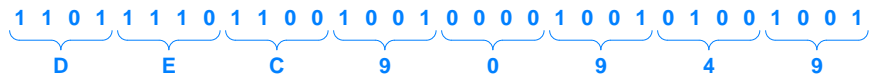
Figure 3.5 Illustration of the relationship between binary and hexadecimal. Each hex digit represents four bits.
