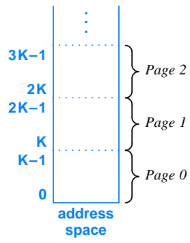
Figure 13.9 Illustration of a virtual address space divided into pages of K bytes per page.
