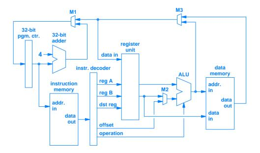
Figure 6.9 Illustration of data paths including data memory.
