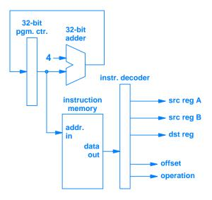
**Figure 6.6** Illustration of an instruction decoder connected to the output of the instruction memory.
