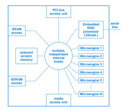
Figure 22.6 Example of a chip-level architecture that shows the major internal components of a Netronome network processor. Access units provide connections outside the chip.
