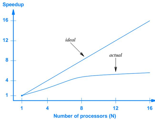
**Figure 18.6** Illustration of the ideal and typical performance of a multiprocessor as the number of processors is increased. Values on the y-axis list the relative speedup compared to a single processor.
