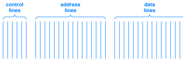
Figure 15.4 Conceptual division of wires that comprise a bus into lines for control, addresses, and data.
